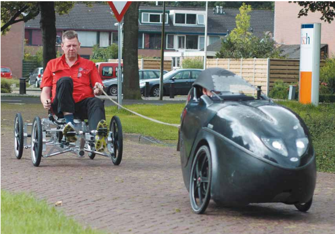
ABOVE: Arjan Vrieling of Flevobike Technology pilots the Prototype 3 chassis, towed behind an electric-assisted Orca velomobile. This could have been to test the suspension response without drivetrain influences – but actually it was because we couldn't wait to test it even before the drivetrain was installed!
